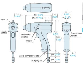
Note: An exclusive intermediate cable (oil-resistant, heat-resistant, flexible type, ø3.7 mm ø0.146 in, 2 m 6.562 ft long) is attached.
